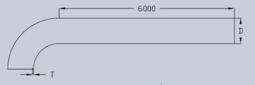
Example: pipe 6 m + curve (curve radius = 1.5 x pipe diameter)Pipe diameter (D):Max wall thickness (T):30 - 300 mm10 mm350 mm8 mm
